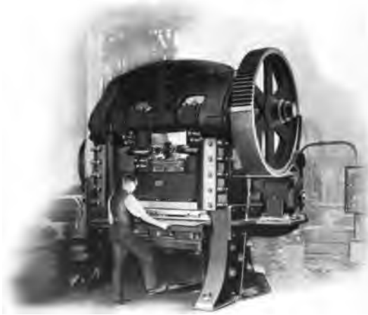
Large Punch driven by a Type C Induction Motor
